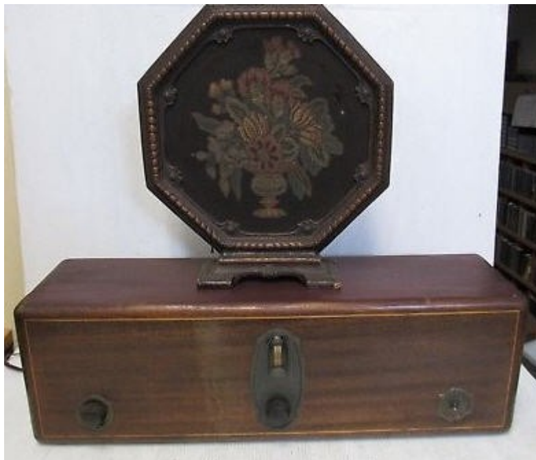
A Radiola 18 which, thanks to Armstrong's simplification of the superheterodyne circuit had only three simple, easy-to-use controls: ON/OFF, Tune, and Volume
